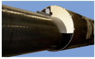
Attach foam segments on the carrier pipe and insert into casing pipe. At this the heightend collar lays on the outside of the face side of the casing pipe. Therefore a secure support is guaranteed.
