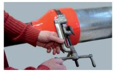
2. Introduce the strap laterally in the clamping tool, push the clamping tool up to the loop, press the holding lever and tighten the strap by turning the crank.
