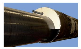
The cable casing pipe has to be pushed between the semicircular cavities. If the cavities are too small they can be slightly enlarged by cutting-out with a knife.
