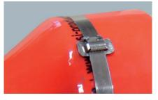
**4.** Cut off the steel strap with the clamping tool cutting lever to immediately obtain the correct length. Immediately strike the cut off end on the stainless steel loop with a hammer. Then bend over both barbs of the loop to protect the strap.
